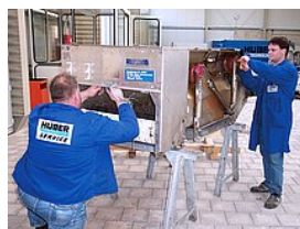
Repair and maintenance of a 3rd party step screen
