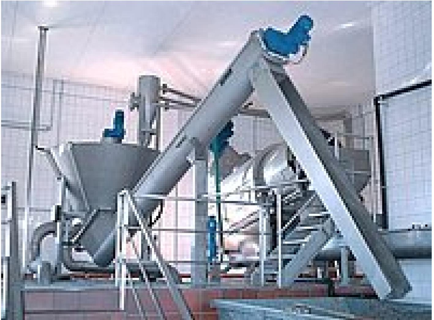
Treatment of grit from wastewater treatment plants and sewer systems by means of a Wash Drum / Grit Washer
