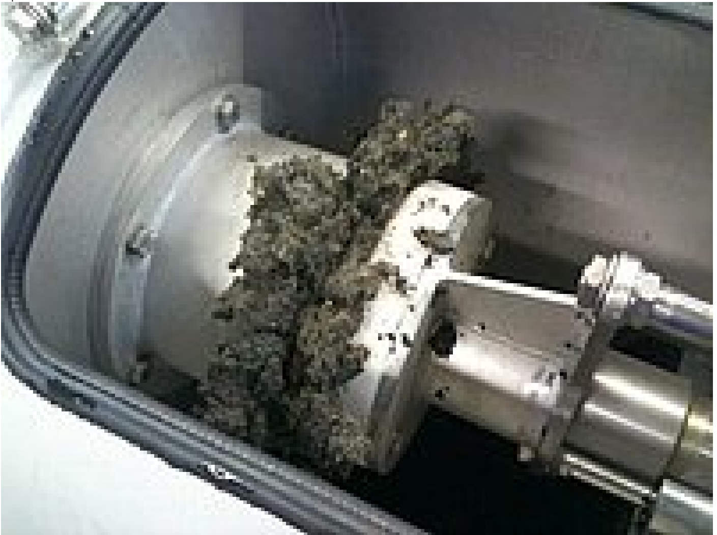
Solid material dewatered to 40% DR by a STRAINPRESS®
