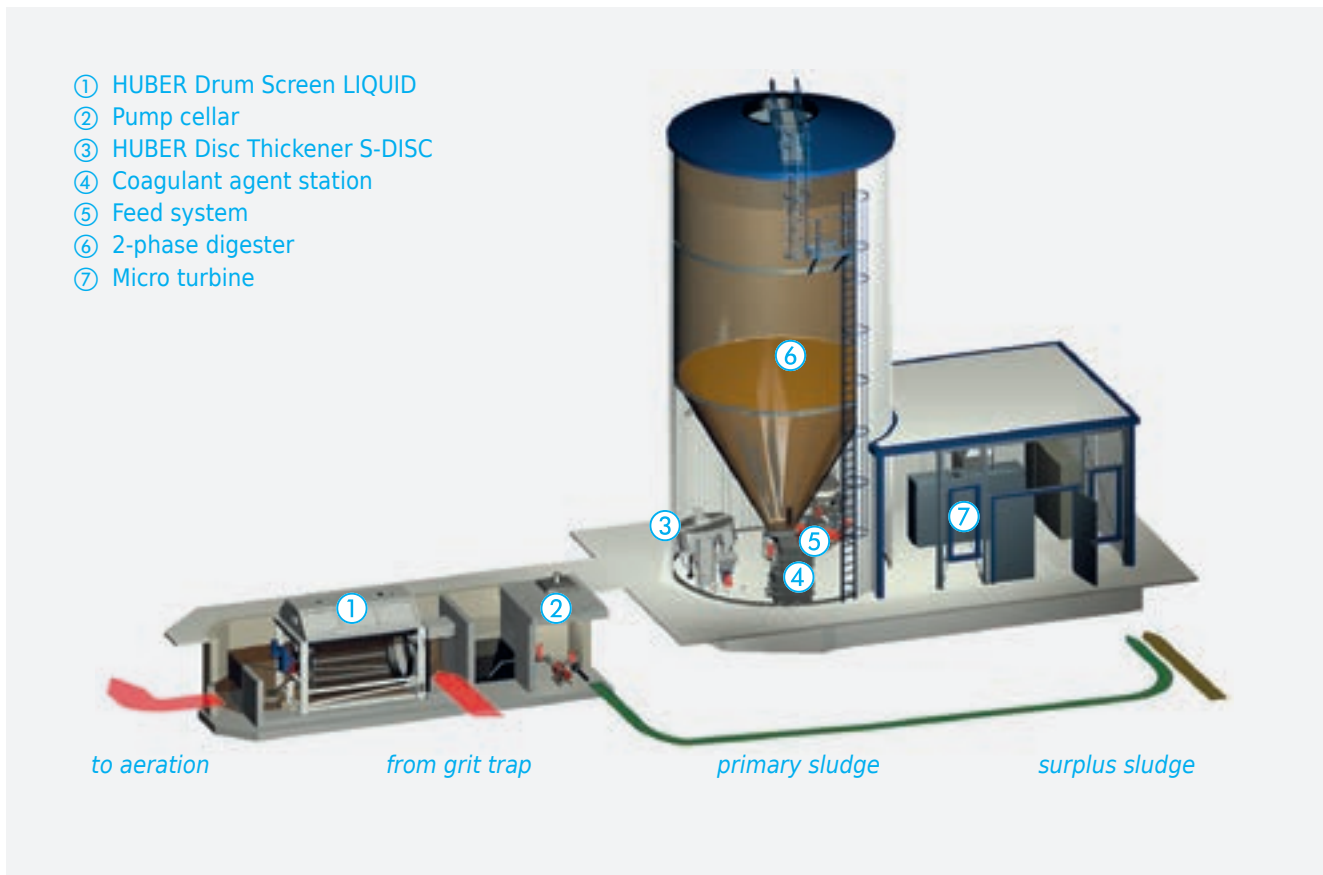
Fig. 6: Process change from aerobic to anaerobic sludge stabilisation with the HUBER CarbonWin® system.
