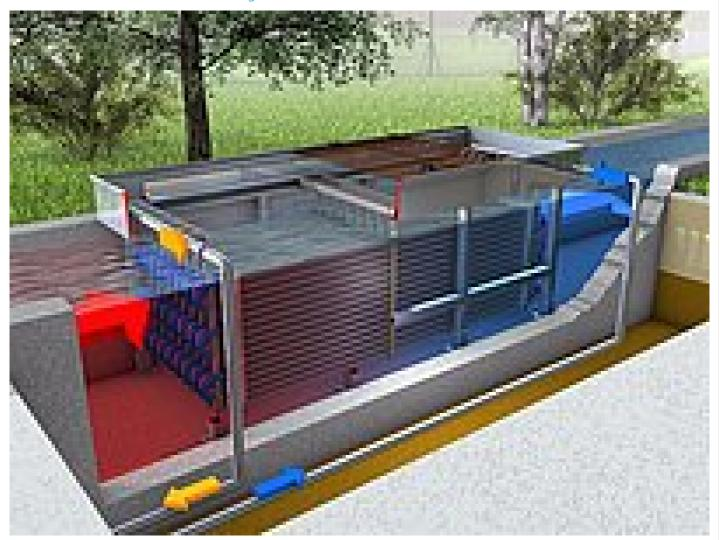
The HUBER Heat Exchanger RoWin is unique of its kind. The wastewater heat exchanger brilliantly combines excellent heat transfer and automatic surface cleaning. A screw ensures automatic removal of sediments. The RoWin heat exchanger can therefore be used for any sort of wastewater, though municipal wastewater is certainly the most frequent application. The 'raw material' wastewater is taken directly from the sewer or downstream of the mechanical treatment stage on the WWTP.
