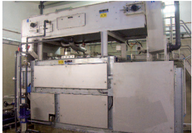
The HUBER Bogenpress can be combined with the Drainbelt unit to further increase capacity
