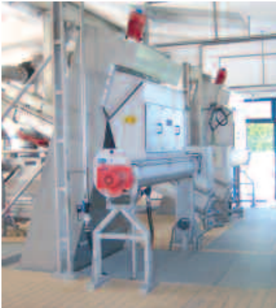
Enclosed STEP SCREEN® SSV for odour-free screenings discharge
