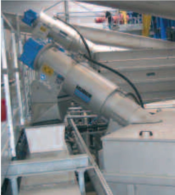
Tank-mounted ROTAMAT® Rotary Drum Fine Screen Ro 2 / RPPS
