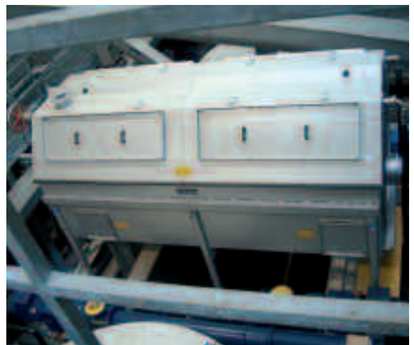
ROTAMAT® Rotary Drum Screen RoMesh® with 0.5 mesh size for wash water recovery
