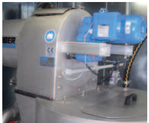
ROTAMAT® Pipestrainer with 0.5 mm wedge wire for removal of fibres
